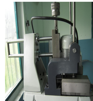
Welding burr remover head riding on hardened spindles
