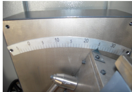
Adjustable grinding angle
