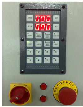
24V Control panel
