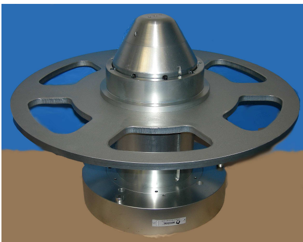
Pneumatic Chuck for internal cores of 8". Expulsion ring and standard lug of L=100mm Automatic back air entrance through the machine.
